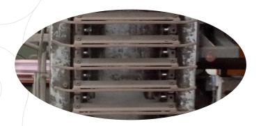
The Delta® treatment prevented the chains from wear as no other treatment did. As the chains were in a matched set of four, they run perfectly together and the customer have had no issues with the chains wearing prematurely. These chains lasted over twice the life of the previous chains! That's why our chains are installed on all the customer's machines.
