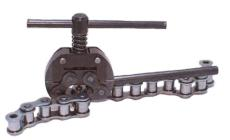
CHAIN EXTRACTOR REF 9130 Simplex, duplex and triplex chains of pitches from 8 to 19,05mm in British and American standards
