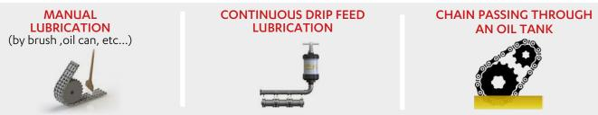
In transmission, any of these methods can be used, although the choice depends on the **type and speed of the chain**. When lifting, manual or continuous drip lubrication is usually employed, although automatic brushes can equally be used.
